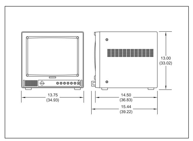
Figure 6. PMC14F Series Dimension Drawing
